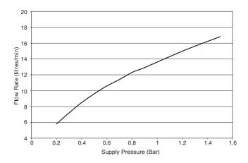
Typical Flow Rates on High Pressure Systems (1 Bar to 5 Bar, with 12 Litre/Min Flow Regulator fitted in shower control outlet) - Mira Silver with L10 Adjustable Fittings or Rigid Head:
